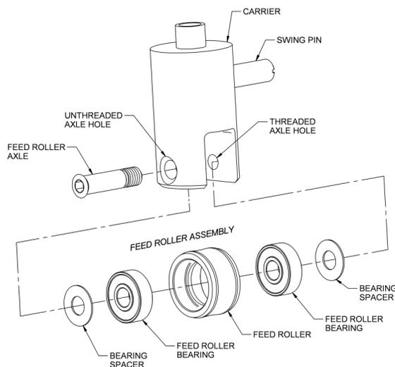
**Note: The Bearing Spacers must be installed between the Carrier and each Feed Roller Bearing (as illustrated) in order to ensure proper operation and to obtain maximum Feed Roller life.**
