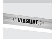
The shaped profile ultra high strength steel booms provide improved rigidity, stiffness and performance
