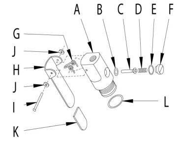
First remove the Capping screw (F). Note that the Valve Stem (C) should be replaced if it is worn and loose in Valve Body (A).
