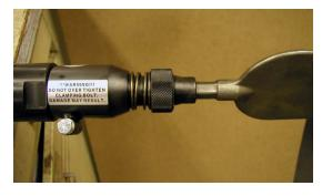
Pictured above shows the chisel installed. To remove a chisel reverse the above procedure and pull the chisel out of the chisel holder.
