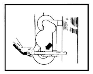
Insert either socket on winch handle onto lower shaft and turn handle counterclockwise to lower load.
